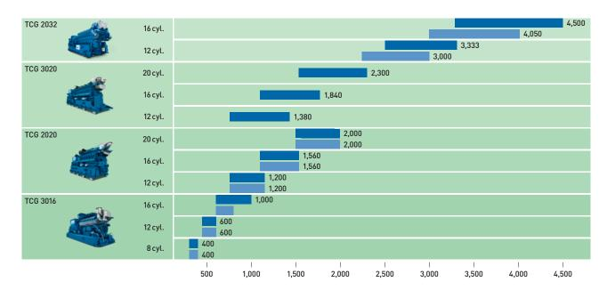
The MWM product portfolio comprises gas engines and gensets in the output range from 400 kW<sub>el</sub> to 4,500 kW<sub>el</sub>. Power plants with an output of 100,000 kW<sub>el</sub> and more are technically feasible.
