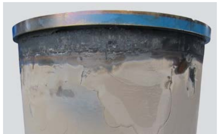
Cylinder liner TCG 2016 after 8000 oh with heavy deposit formation due to an incorrect inhibitor dosage
