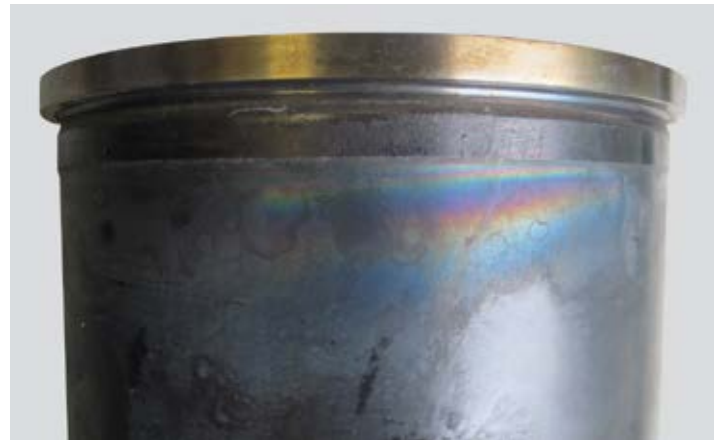
Cylinder liner TCG 2016 after 10,000 oh with MWM Premium Antifreeze -20
